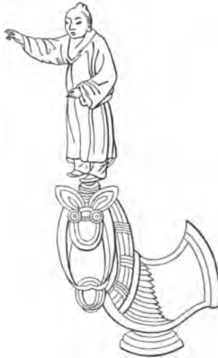
A CHINESE MAGNET-FIGURE, AS USED IN SHIPS OF EIGHTH AND NINTH CENTURIES A.D.
