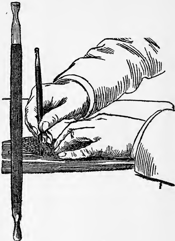
FIG. 27.—SECOND POSITION OF OUTLINING TOOL
