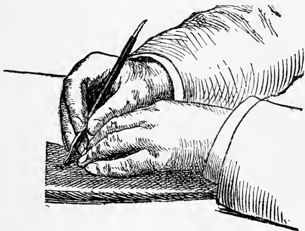
FIG. 26.—FIRST POSITION OF OUTLINING TOOL
