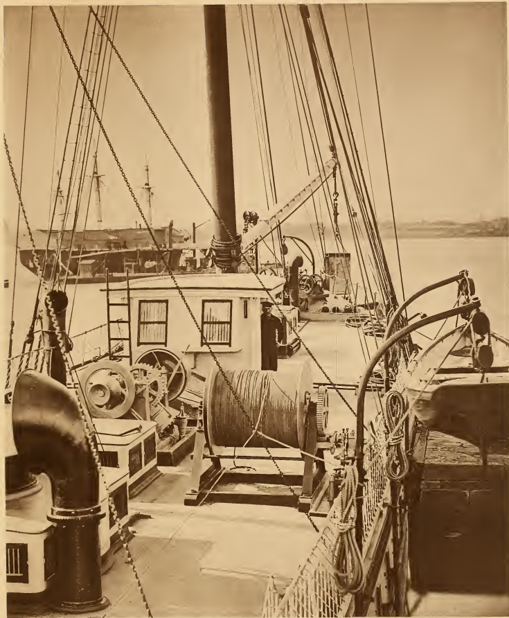
VIEW OF THE "BLAKE'S" DECK LOOKING FORWARD FROM THE BOW OF THE STARBOARD QUARTER-BOAT. READY FOR PAYING OUT THE DREDGE.
