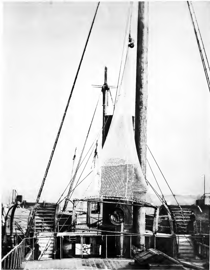
THE IMPROVED TRAWL SHOWN AS HAVING "TRIPPED" AFTER FOULING WITH ROUGH BOTTOM.
