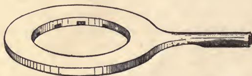
FIG. 7.—Annular ventilating-tube over bowl.
