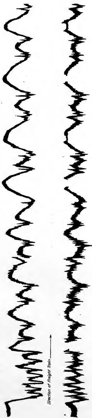
Fig. 23—Photographic Records of Movement at Joint. Upper Record Magnifies Movement 3.79 Times; Lower Record, 3.91 Times.
