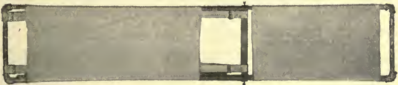
FIG. 68.—The Gas-Pipe Frame, with canvas stretched over it, and sanitary aperture (Bradford and Lovett).
