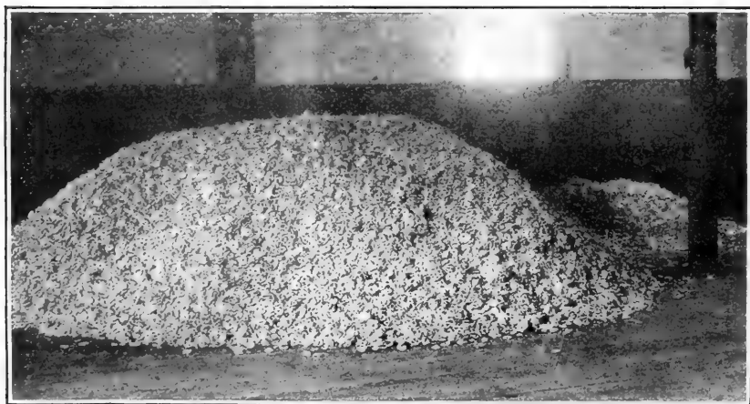
FIG. 14.—A pile of evaporated apples going through the sweating process in a curing room connected with a New York evaporator.
