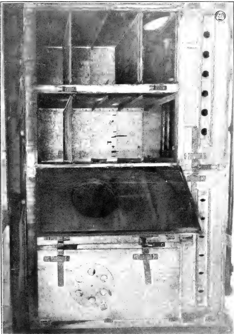
STEAM OVEN USED AT THE FOREST PRODUCTS LABORATORY FOR DRYING MOISTURE SECTIONS. THE THERMOMETER, SHELVES, AND A PORTION OF THE HEATING COILS CAN BE SEEN IN THE OPEN SECTIONS.
