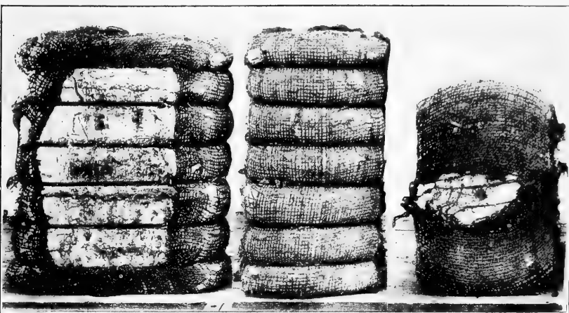
FIG. 1.—FLAT OR UNCOMPRESSED BALE, TOP, SIDE, AND END VIEWS. DENSITY, 12 TO 15 POUNDS PER CUBIC FOOT. APPROXIMATE DIMENSIONS, 54 BY 27 BY 48 INCHES.
