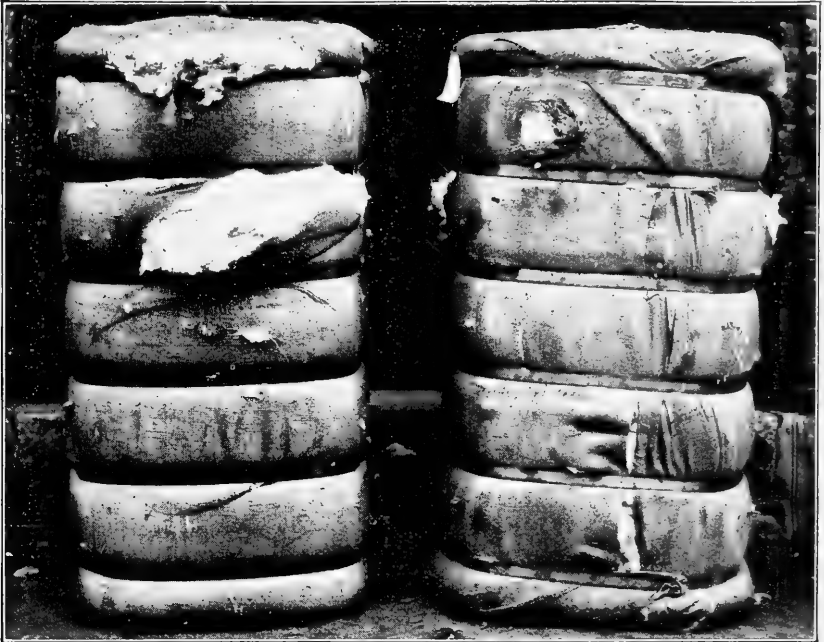
GINNER'S COMPRESS BALE, SHOWING TOP AND SIDE OF BALE. DENSITY, 25 TO 35 POUNDS PER CUBIC FOOT. APPROXIMATE DIMENSIONS, 52 BY 25 BY 20 INCHES.
