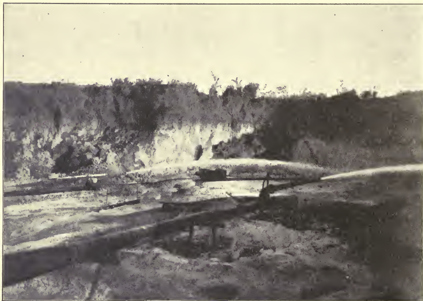
FIG. 275.—Hydraulicking at the Gopeng tin mine, Perak. Wolf.
