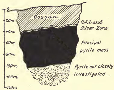
FIG. 12.—Vertical section of No. 2 ore-body, Rio Tinto, illustrating secondary depth-zones in the case of cupriferous pyrite carrying a little gold and silver. Vogt, Zeit. f. prakt. Geol. , 1889, p. 250.
