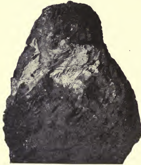
FIG. 92.—Secondary silver (bright) upon the cleavage-planes of galena from the cementation zone.
