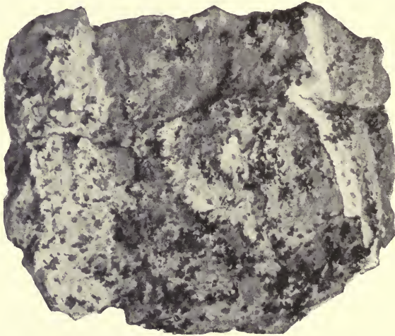
FIG. 90.—Spots of cinnabar in Carboniferous sandstone, the result of both pore-filling and metasomatic replacement. Nikitovka. Ekaterinoslav. Collection, Geol. Landesanst. , Berlin.
