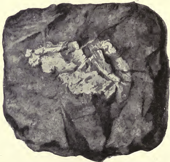
FIG. 99.—Bornite, metasomatically replacing chalcopyrite represented by the light core in the centre. Monte Catini, Val di Cecina, Tuscany. Collection, Geol. Landesanst. , Berlin.
