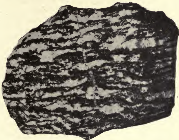
FIG. 122.—Magnetite (dark) and calcite (light) arranged in a banded structure produced by the replacement of certain peculiarly susceptible limestone layers. Schniiedeberg in Silesia. Collection, Geol. Landesanst. , Berlin.
