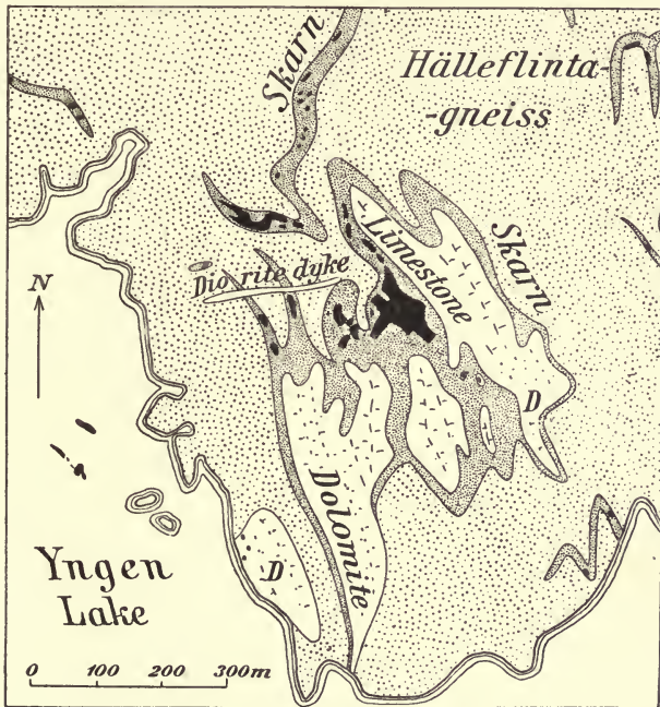
FIG. 246.—Map of the principal portion of the Persberg field ; ore and workings indicated black. Törnebohm.
