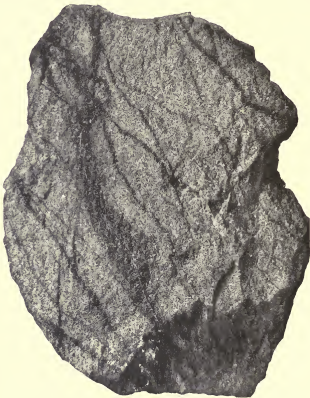
FIG. 267.—Cassiterite veins and greisen in the Altenberg granite.
