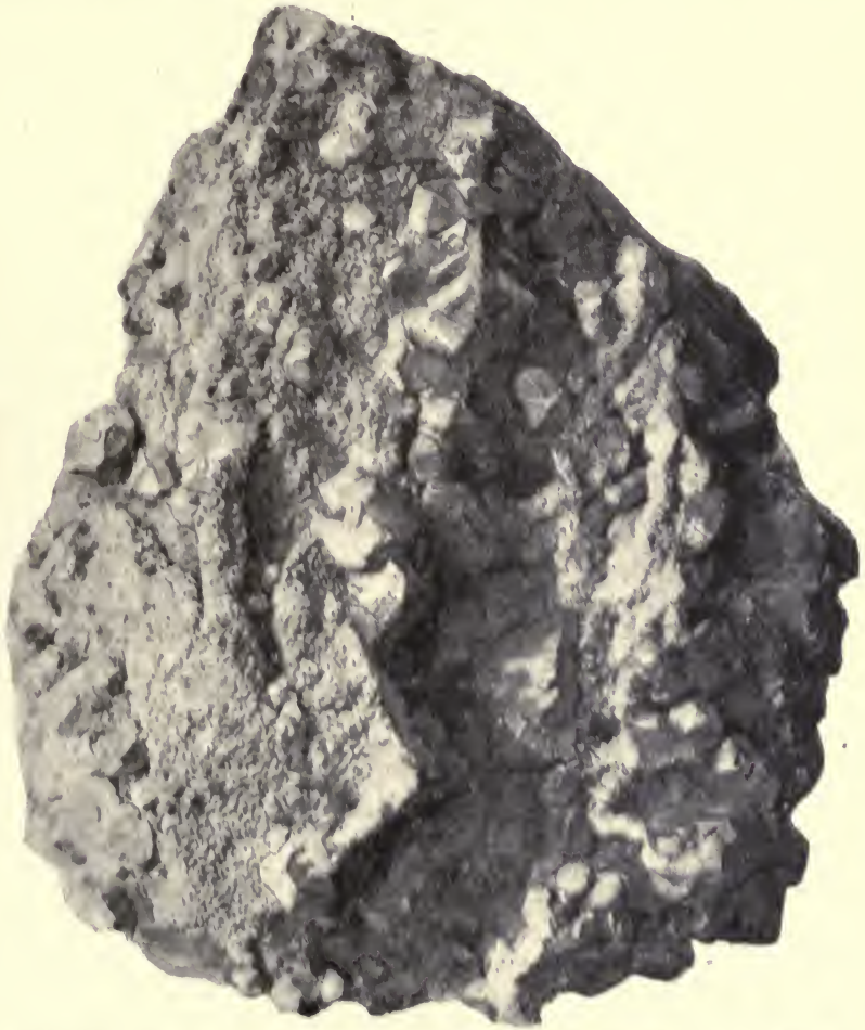
FIG. 131.—Primary drusy structure resulting from the incomplete filling of a fissure. Glückauf mine, near Velbert, Westphalia. Collection, Geol. Landesanst. , Berlin.
