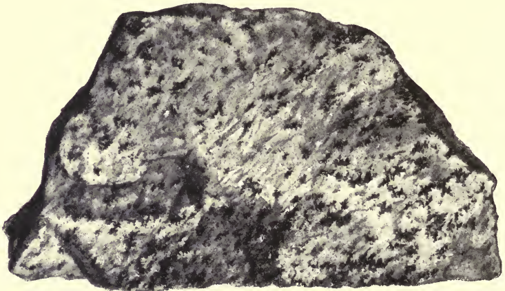
FIG. 111.—Cassiterite (dark) disseminated in greisen; primary ore from Geyersberg near Geyer. Collection, Geol. Landesanst. , Berlin.
