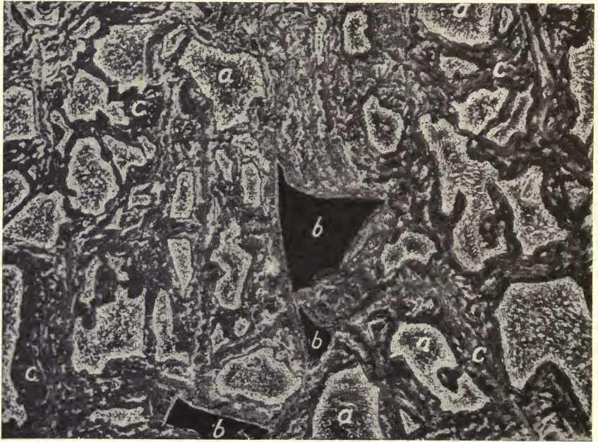
FIG. 96.—Chalcopyrite, at the junction of the oxidation zone with the cementation zone, in process of decomposition to cuprite and malachite. Boliver, Santander, Columbia. Magnified 18 times.
