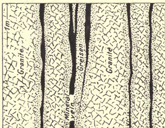
FIG. 145.—Granite altered to greisen along mineral veins. Telemarken, Norway.
