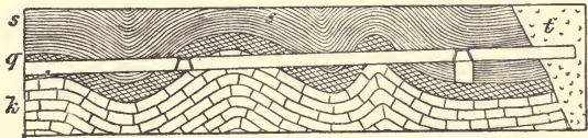
g, Quartzose bedded mass containing antimony ore; k, Limestone; s, Clay-slate; t, Trachyte.
