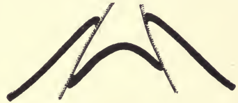
FIG. 29.—Two overthrusts dipping away from one another, the portion of deposit between them remaining unmoved at a lower level.
