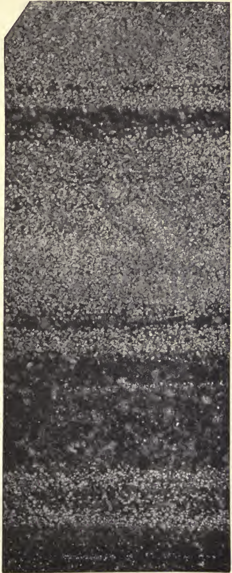
FIG. 4.—Pyritic band from the Witwatersrand, showing pyrite layers, light in colour, with quartzite layers, dark in colour, the composition of these layers differing only quantitatively. Voit, Zeit. f. prakt. Geol. , 1903, p. 216.
