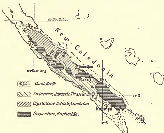
FIG. 156.—Distribution in New Caledonia of the serpentine rock carrying the veins of garnierite and asbolane.
