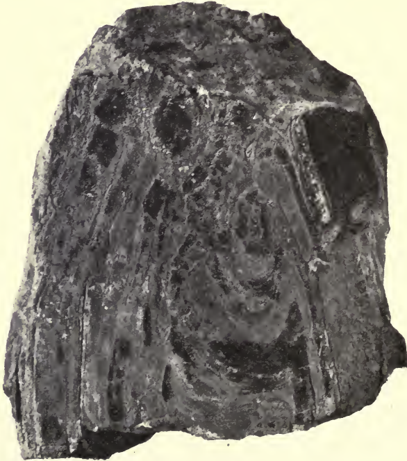
FIG. 121.—Banded structure with ore-beds. Itabirite from Krivoi Rog, South Russia, consisting of alternating beds of quartz (light) and hæmatite (dark). Collection, Geol. Landesanst. , Berlin.
