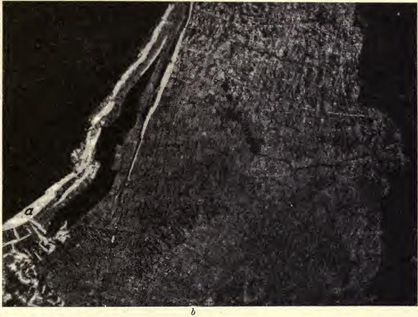
FIG. 139.—Metallic silver as white streaks ( a ), deposited along the cleavage-planes of galena ( b ). Mexico. Magnified 18 times. Collection, Geol. Landesanst. , Berlin.
