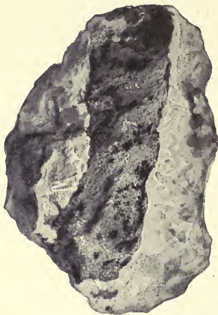
FIG. 104.—Smaltite vein (dark) containing niccolite (dark grey) and smaltite (light grey), and itself contained in dolomite and calcite. Hydrochemical filling. Cobalt, Canada. Collection, Geol. Landesanst. , Berlin.
