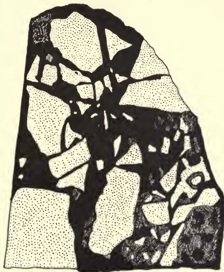
FIG. 193.—Ore breccia from Mertainen consisting of fragments of syenite-porphry cemented by magnetite. W. Petersson.
