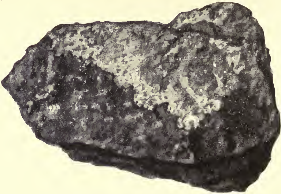
FIG. 110.—Cassiterite (dark) and stanniferous pyrite (light). Primary ore from the Bolivian lodes. Avicaya, North Bolivia. Collection, Geol. Landesanst. , Berlin.
