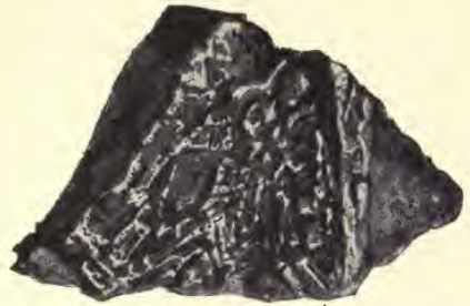
FIG. 106. — Niccolite (light) magmatically separated in a mixture of plagioclase and augite. Los Jarales near Caratraca, Malaga. Collection, Geol. Landesanst., Berlin.
