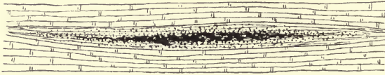
FIG. 66.—Diagram of a fahlband showing the relation between the metalliferous lens and the whole bed.
