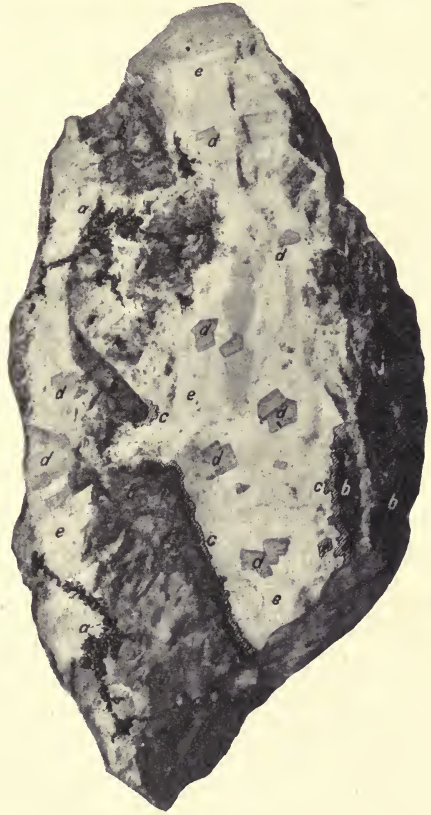
FIG. 256. — Specimen from Kupferberg in Silesia with characteristic chlorite gangue and felspar; one-quarter natural size. Collection, Geol. Landesanst., Berlin.
