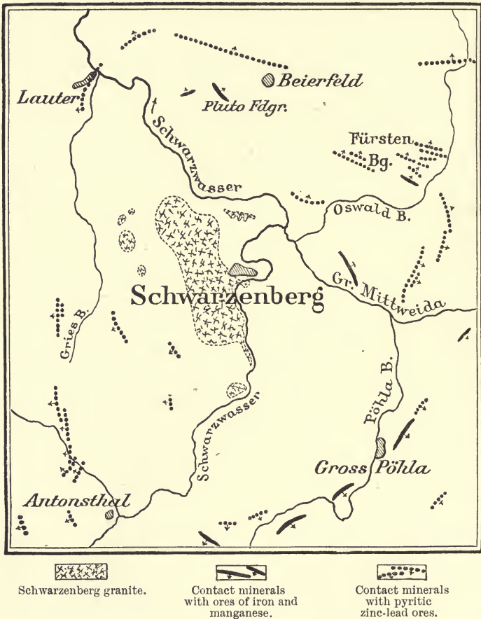
FIG. 47.—Ore-deposits in the granite contact-zone at Schwarzenberg in Saxony. Blatt Schwarzenberg der Geol. Speciale Karte.
