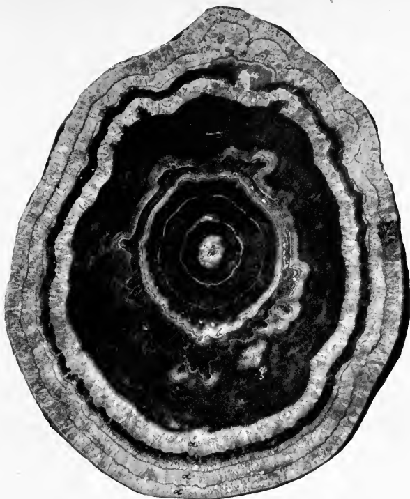
FIG. 125.—Concentric crusted structure of marcasite ( a ), with dark- and light-coloured schalenblende ( b ). Schmalgraf mine, near Aachen. 1.5 times less than natural size. Collection, Geol. Landesanst. , Berlin.
