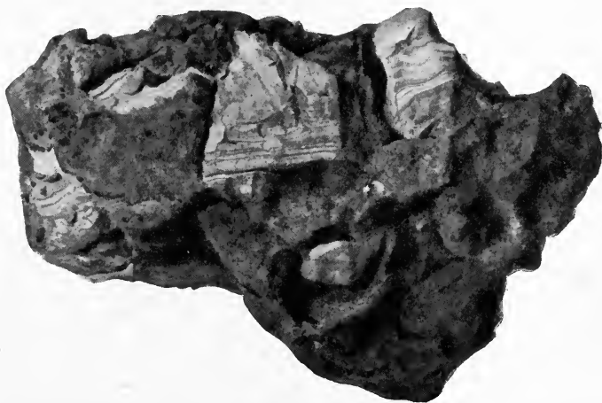
FIG. 94.—Metasomatically formed schalenblende (white with grey stripes) altered, except for some fragments, to smithsonite. Oxidation zone of the Schmalgraf mine near Aachen. Collection, Geol. Landesanst. , Berlin.
