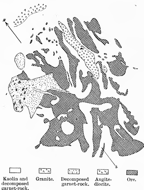
FIG. 236.—Horizontal projection through the Dalnaia mine. Scale, 1:1700. Tscherm. Min. u. Pet. Mitt. Vol. XXIII., plate 4.
