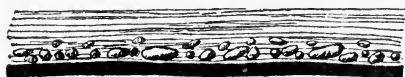
FIG. 62.—Clay ironstone concretions in the hanging-wall of the main seam in the lean portion of the Westphalian coalfield; these concretions, containing Goniatites , represent a marine horizon.
