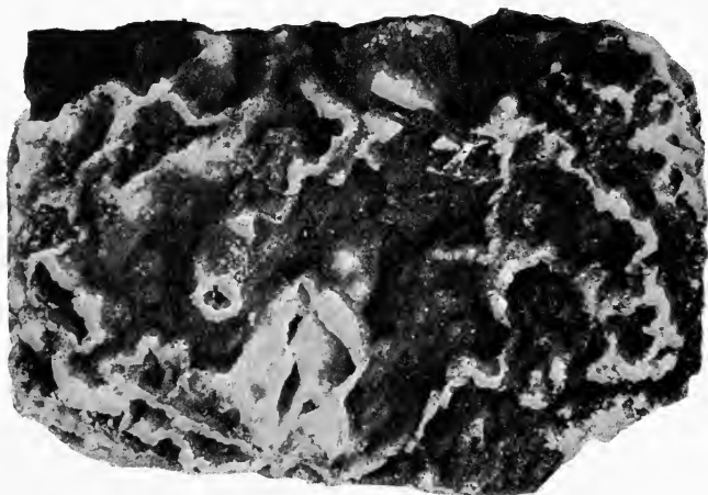
FIG. 133.—Drusy structure resulting from the removal of some of the original components by solution, quartz remaining. Spital Lode, Schemnitz. Collection, Geol. Landesanst. , Berlin.
