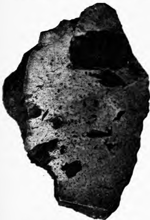
FIG. 129.—Brecciated structure. Fragments of slate torn from the country-rock and enveloped in a magmatic deposit of pyrrhotite. Mug mine, Norway. Collection, Geol. Landesanst. , Berlin.
