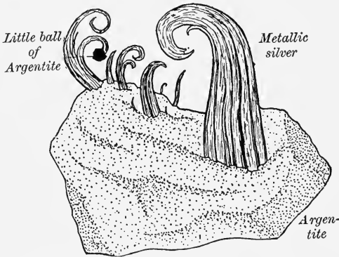
FIG. 140.—Horns of metallic silver arising from argentite. Vogt, Zeit. f. prakt. Geol. , 1899, p. 115.
