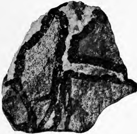
FIG. 128.—Brecciated structure. Fragments of arkose sandstone cemented by sphalerite (dark) and quartz (light). Schauinsland mine, Black Forest. One-half natural size. Collection, Geol. Landesanst. , Berlin.
