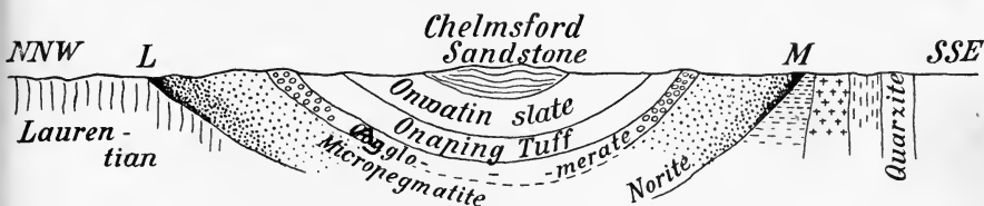
FIG. 199.—Diagrammatic section of the Sudbury field. Coleman, 1907.
