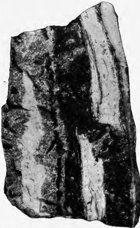
FIG. 69.—Kink in a newly opened pyrite vein in a lode. Traugott lode. Freiberg district. Two-thirds natural size.
