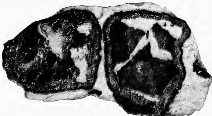
FIG. 126.—Concentric crusted structure. Fragments of country-rock cemented by quartz and each enveloped in an inner ring of galena (light) and an outer ring of sphalerite (dark). Burgstadt lode-series, Clausthal. Collection, Geol. Landesanst. , Berlin.
