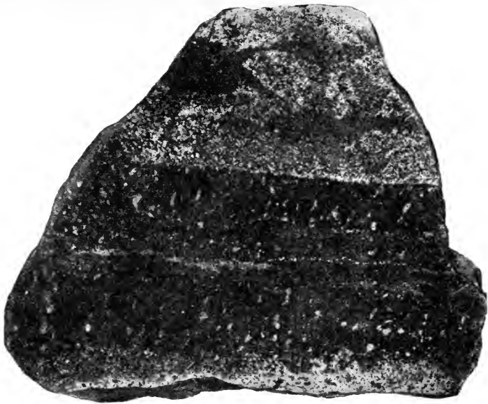
FIG. 120.—Banded structure formed by magmatic segregation. Two bands of pyrite (light) separated by eruptive rock in which nests of chalcopyrite are contained. Nieder-Sohland, Saxony. Magnified 2.5 times. Collection, Geol. Landesanst. , Berlin.
