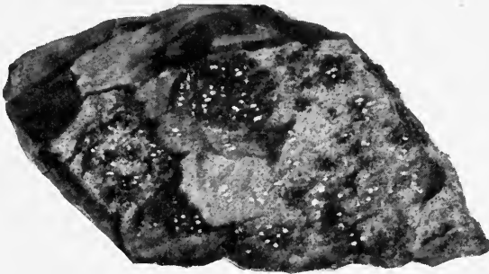
FIG. 109.—Chromite (dark) with specks of niccolite (white spots) in serpentine at Santa de Aguas, Malaga. Collection, Geol. Landesanst. , Berlin.
