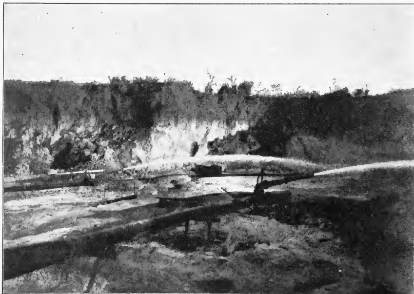
FIG. 275.—Hydraulicking at the Gopeng tin mine, Perak. Wolff.
