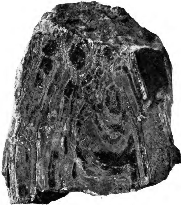
FIG. 121.—Banded structure with ore-beds. Itabirite from Krivoi Rog, South Russia, consisting of alternating beds of quartz (light) and hæmatite (dark). Collection, Geol. Landesanst. , Berlin.
