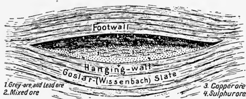
FIG. 164.—Change in the composition of the Rammelsberg ore-bed from the hanging-wall to the foot-wall, considered to be a primary variation.
