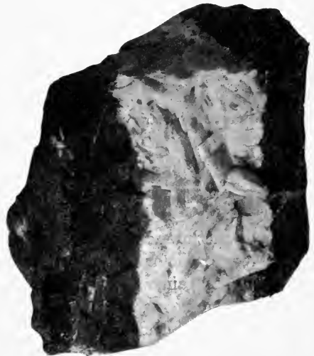
FIG. 123.—Symmetrical crusted structure of chalcopyrite (dark) and calcite (white) in hornblende-schist (grey) from Kupferberg in Silesia. One-half natural size. Collection, Geol. Landesanst. , Berlin.
