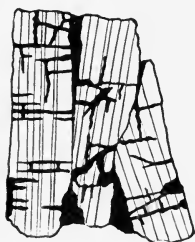
FIG. 195. — Plagioclase crystals from the pyrrhotite-gabbro of the Flaad mine in Norway, traversed by pyrrhotite veins. Vogt, Zeit. f. prakt. Geol. , 1893, p. 139.
