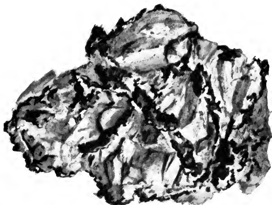
FIG. 97.—Native copper along cracks in quartz; from the oxidation zone, Ocaruzawa, Rikuchu, Japan. Collection, Geol. Landesanst. , Berlin.
