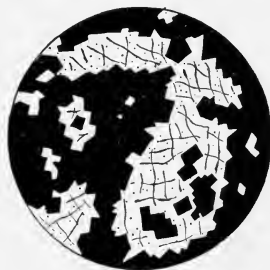
FIG. 168.—Chromite-dunite, consisting of chromite and olivine. Ramberget near Hestmandö; magnified 40 times. Vogt, Zeit. f. prakt. Geol. , 1894, p. 391.
