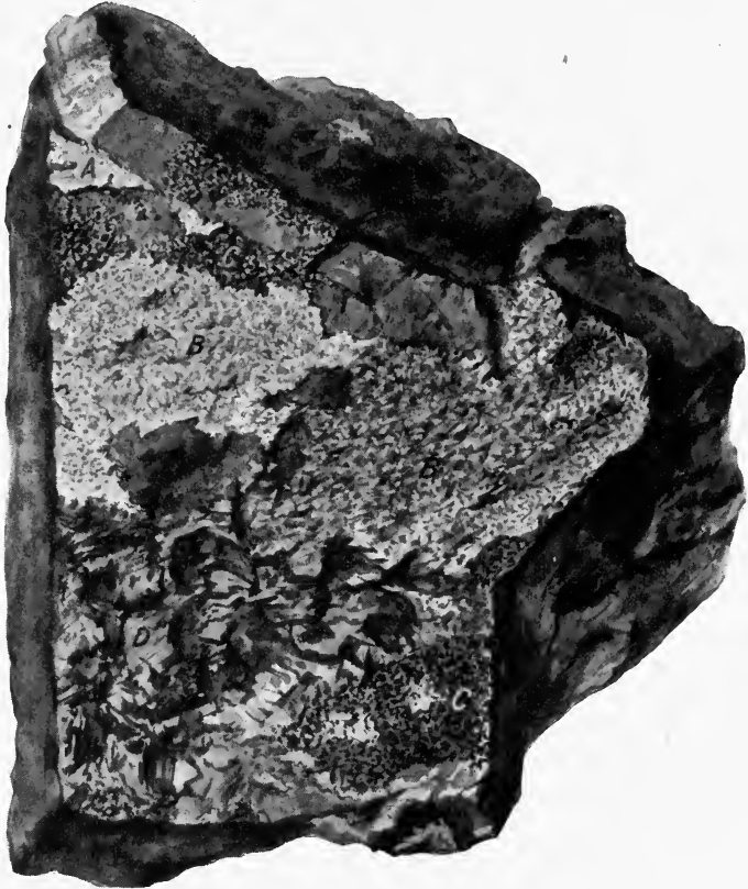
FIG. 87.—Free gold (a), calaverite (b), copper ore (c), and petzite (d), from the Lake View Mine Kalgoorlie. Collection, Geol. Landesanst. , Berlin.
