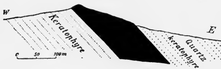
FIG. 191.—Section of the Kiirunavaara deposit through one of the summits of the range.
