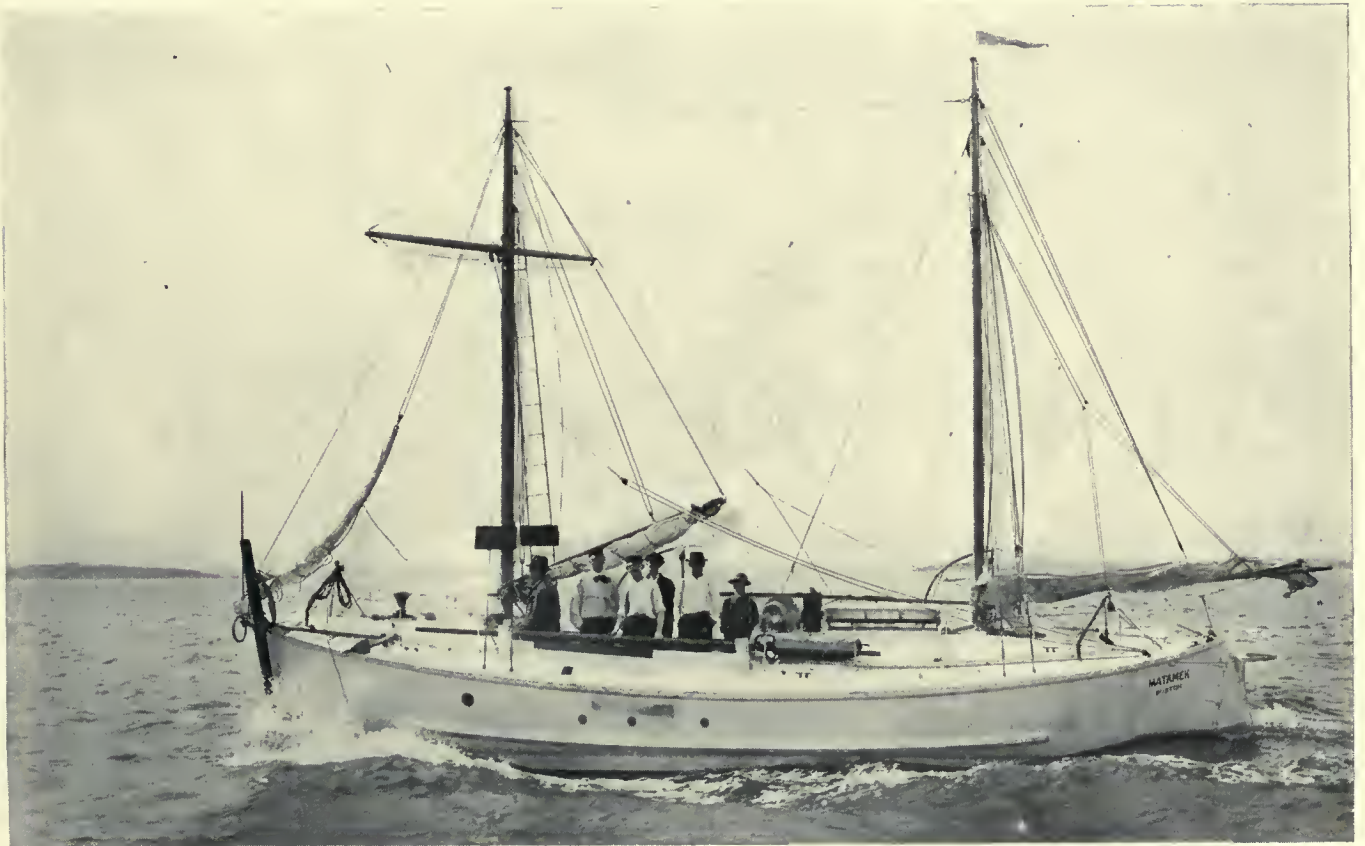
MATAMEK—OWNED BY COPLEY AMORY, OF CAMBRIDGE, MASS. Used in Labradore; 36 feet long by 8 feet 9 inches beam; driven by Lawley 2-cylinder, 4-cycle engine
