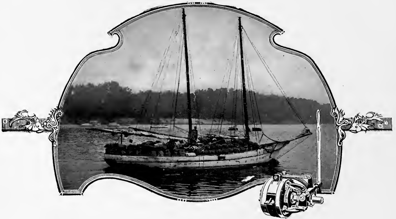
"ELIZABETH C." of Greenport, N. Y. A 16 ton Auxiliary Schooner owned by Capt. S. B. Bushnell. Carrying a cargo of 200 bushels of potatoes. Mainpower plant four cylinder 40 H. P. Frisbie engine equipt with a Paragon Reverse Gear. In service seven years.
