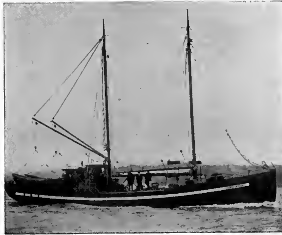
HALIBUT SCHOONER CONSTANCE One of the finest boats ever built for halibut service—She measures 87 feet on deck, 18 feet beam and carries 140 horsepower Standard-Frisco engine
