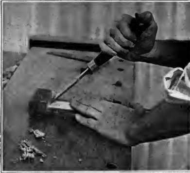
Fig. 41. Trimming a miter.
