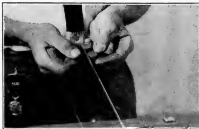
Fig. 86. Breaking the glass. (Step 3.)
