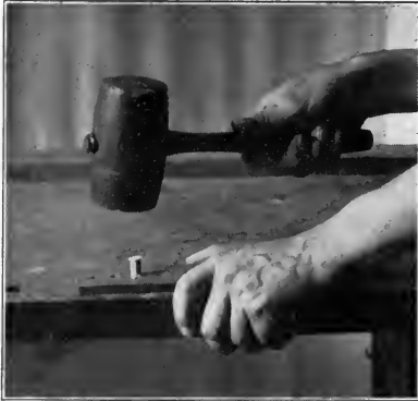
Fig. 132. Driving dowel thru dowel-plate.
