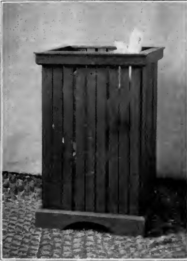
Fig. 10. Basket with mitered frames at top and bottom.
