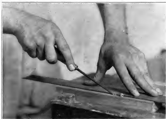
Fig. 176. Guiding a veining tool along a straight edge.
