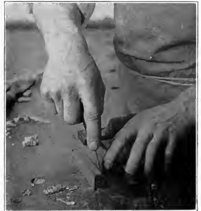
Fig. 35. Scoring with a knife along the try-square.
