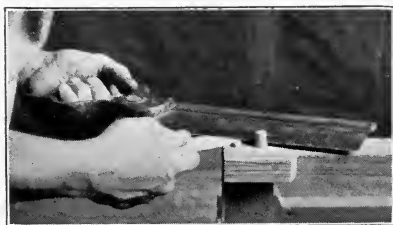
Fig. 139. Sawing off projecting end of dowel-pin.
