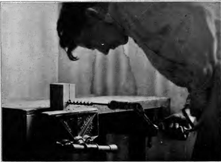
Fig. 156. Boring hole in head of mallet.
