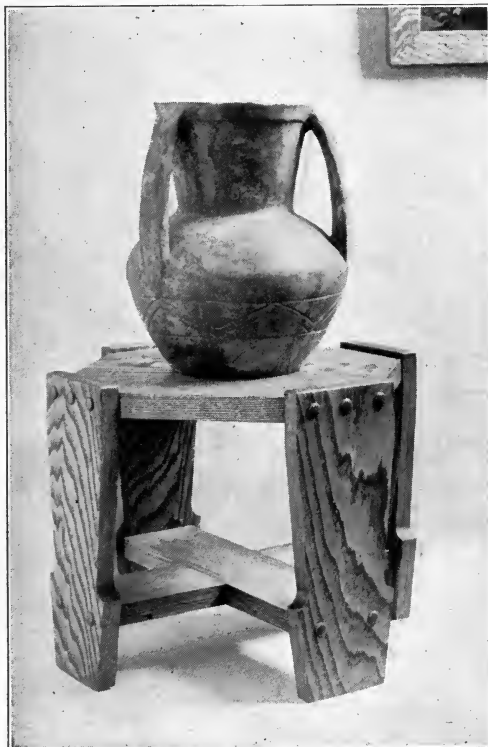
Fig. 142. Dowel ends covered with upholstery nails.
