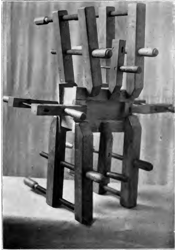
Fig. 192. Gluing the top on to the box.
