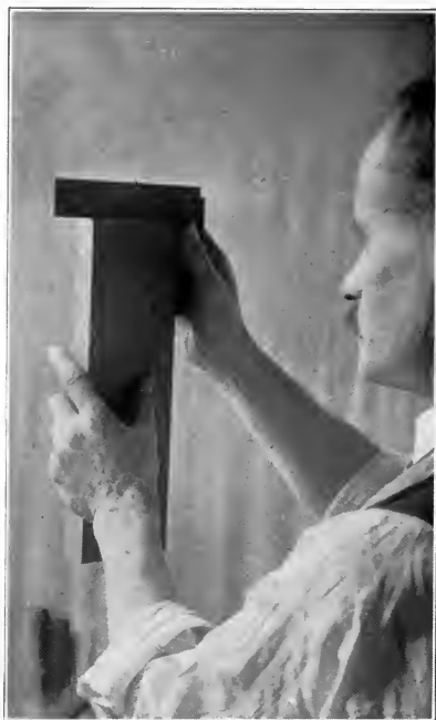
Fig. 27. Testing squareness of end.
