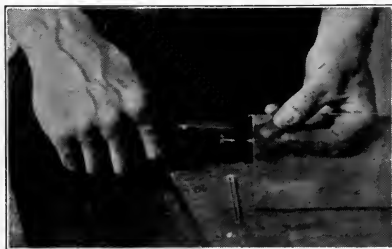
Fig. 87. Breaking off a narrow piece of glass with the pliers.
