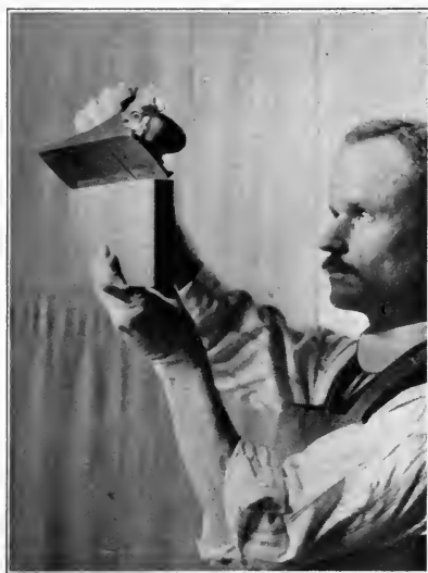
Fig. 23. Testing the straightness of an edge with the arris of the plane.
