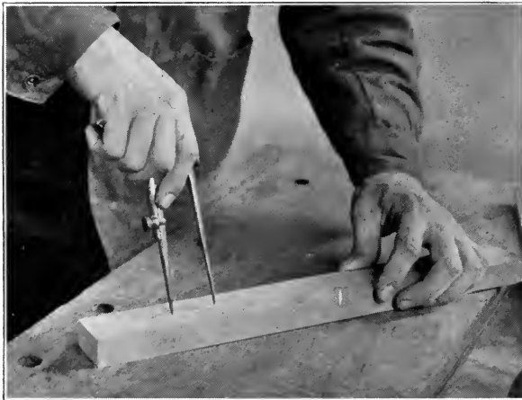
Fig. 58. Stepping off distances with the dividers
