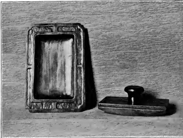
Fig. 174. Tray and blotter with tool marks of gouge left showing.
