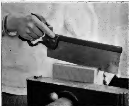
Fig. 193. Sawing the box apart.
