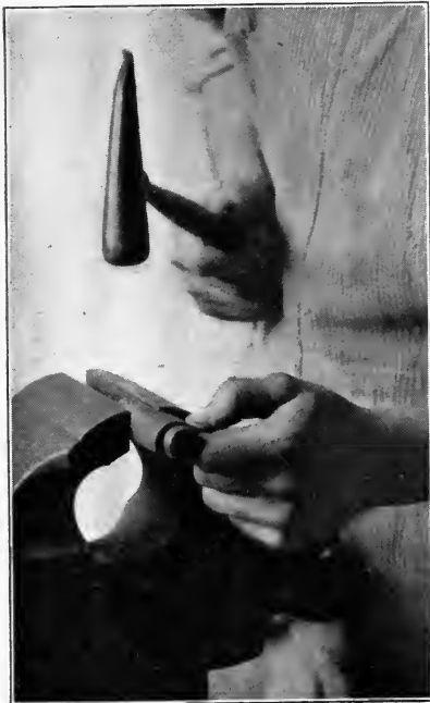
Fig. 108. Hammering a strip into a cylinder.
