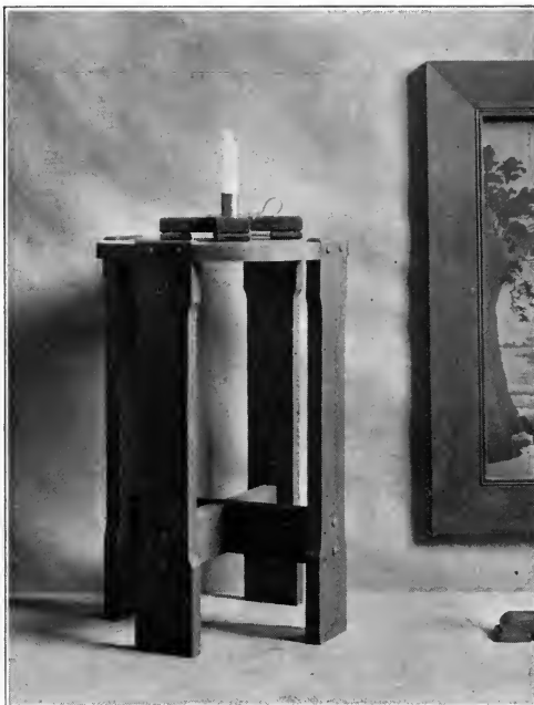
Fig. 145. Legs doweled directly into top.
