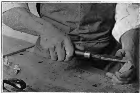
Fig. 33. Slicing off an arris with a chisel.
