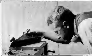
Fig. 34. Testing a planed surface for flatness by using the aris of the plane.
