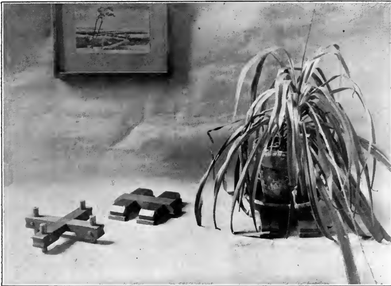
Fig. 120. Flowerpot-stands, made with half-lap joint.
