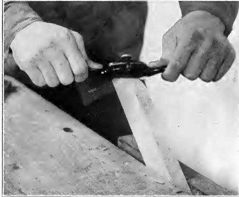
Fig. 57. Using the spokeshave.
