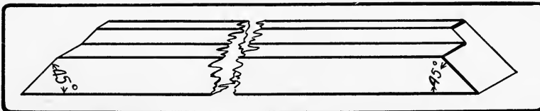
Fig. 79. Rabbeted and mitered member of picture-frame.
