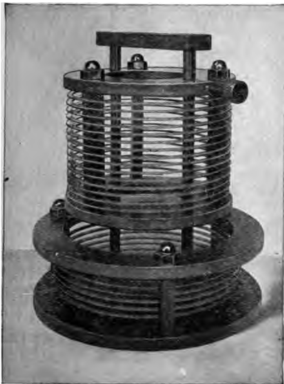
Fig. 31. —An Excellent Example of the Oscillation Transformer, from the International Radio Company.
