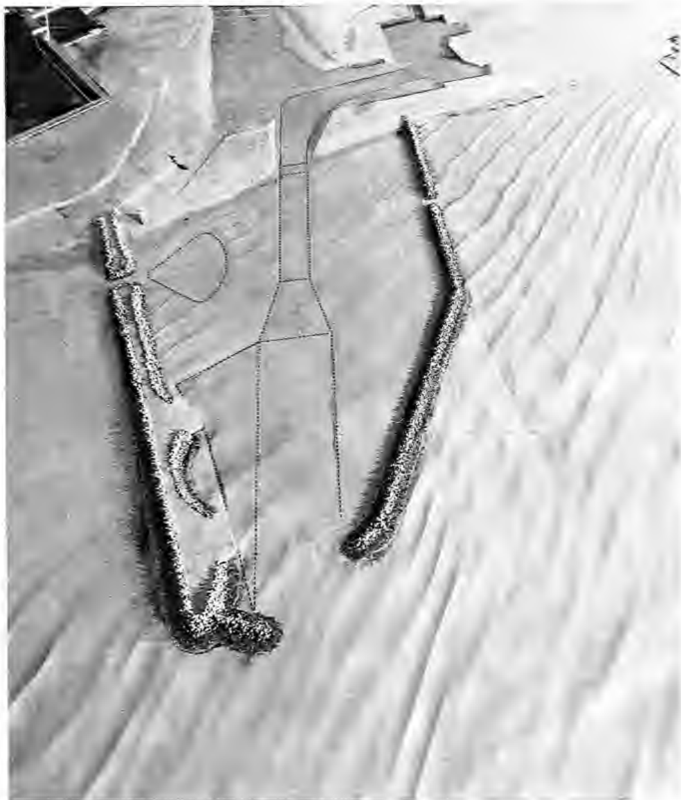
Photo 7. Typical wave patterns for Plan 19; 9-sec, 2-m (6.6-ft) waves from 137 deg; swl = +0.5-m (+1.6-ft)
