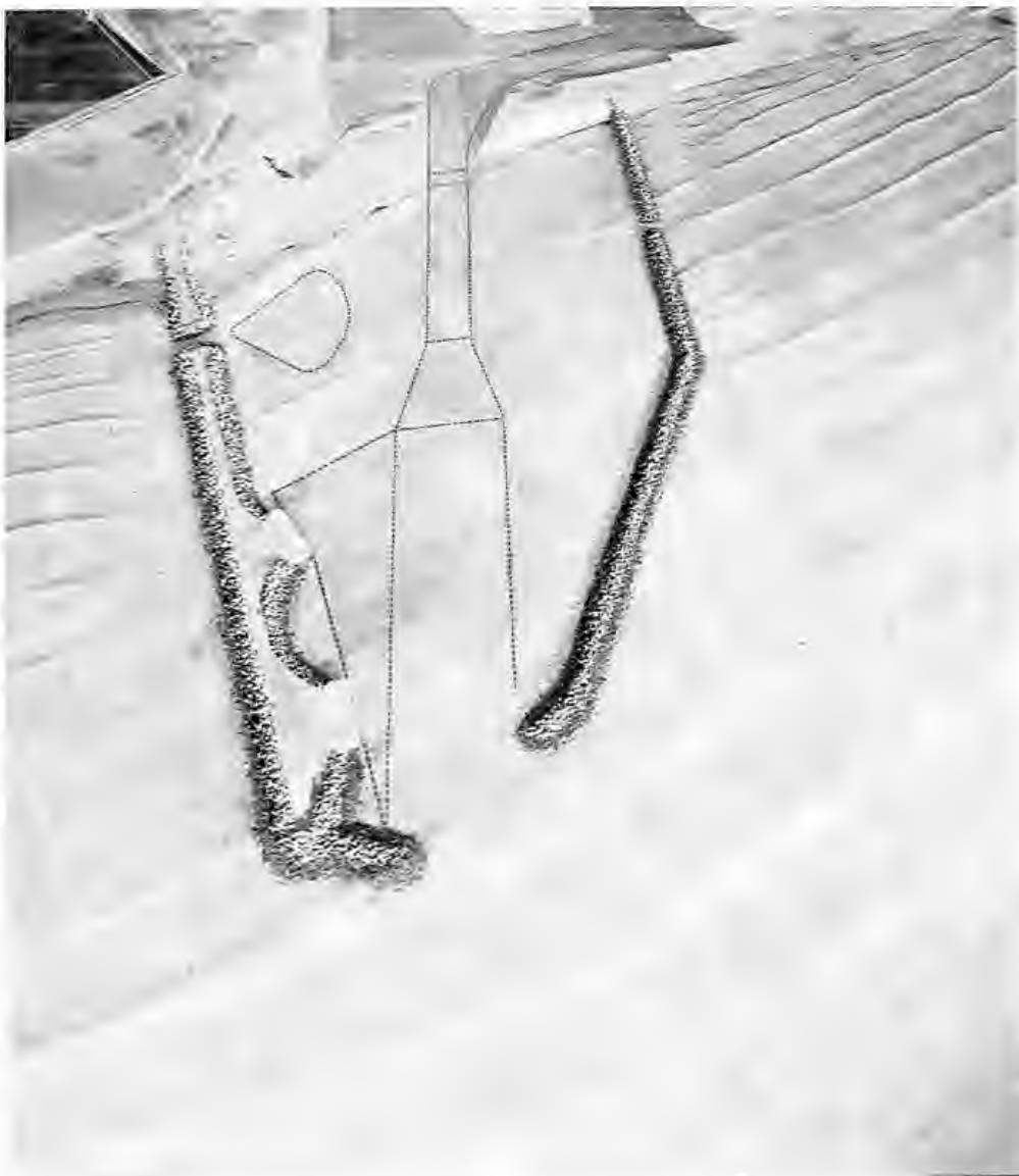
Photo 5. Typical wave patterns for Plan 19; 12-sec, 1-m (3.3-ft) waves from 182 deg; swl = +0.5-m (+1.6-ft)
