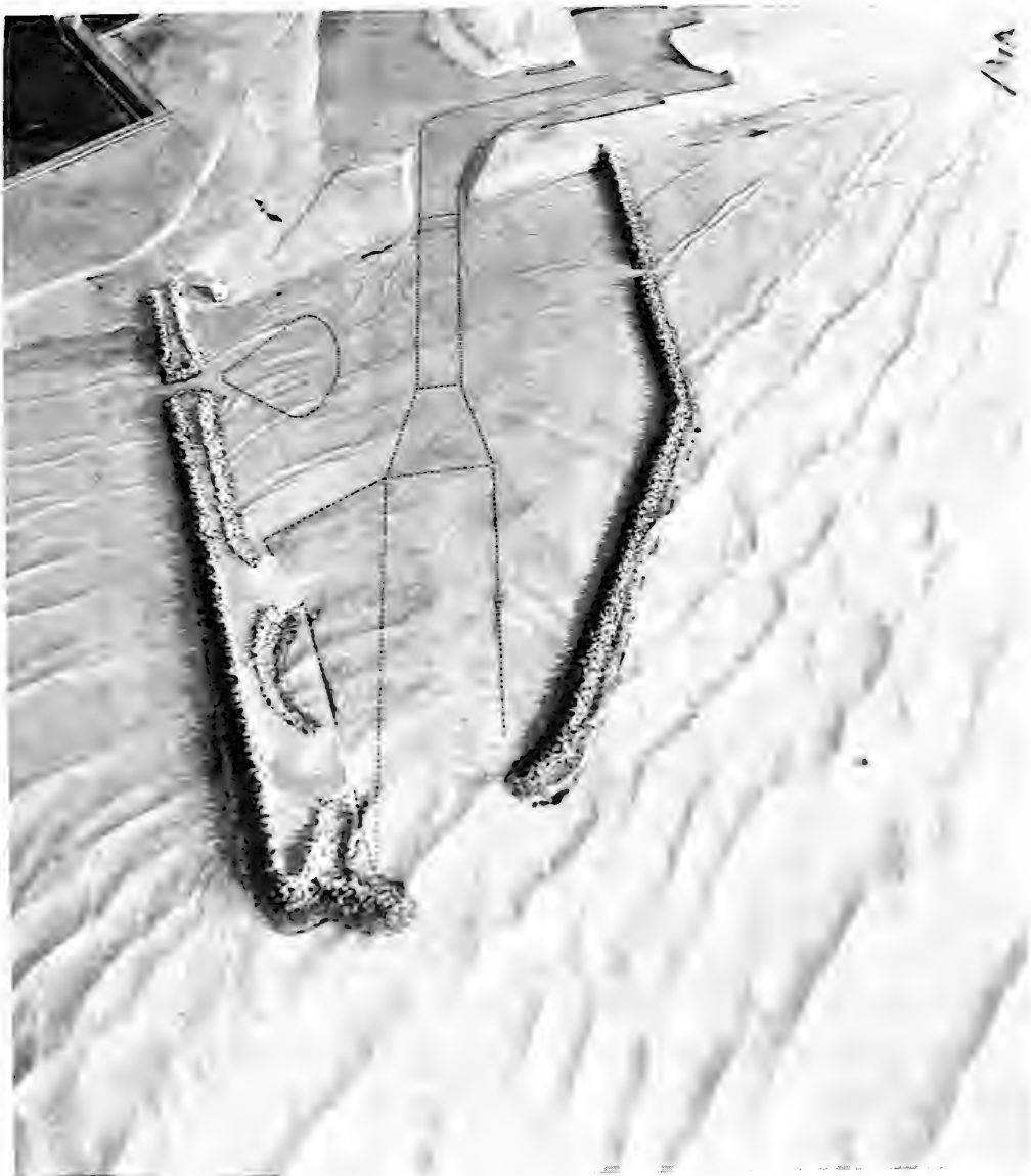
Photo 9. Typical wave patterns for Plan 19; 12-sec, 5-m (16.4-ft) waves from 137 deg; swl = +0.5-m (+1.6-ft)
