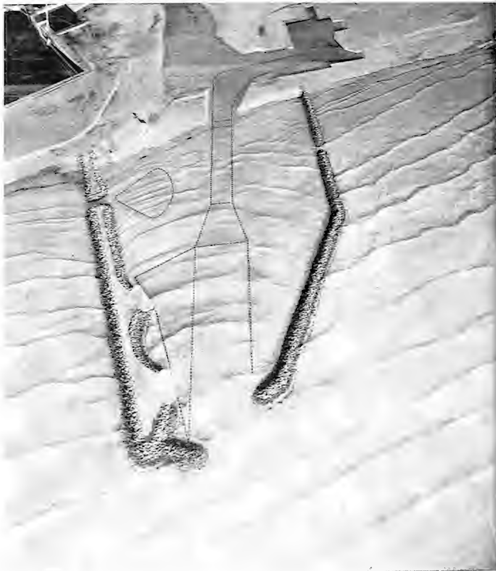
Photo 6. Typical wave patterns for Plan 19; 12-sec, 5-m (16.4-ft) waves from 182 deg; swl = +0.5-m (+1.6-ft)
