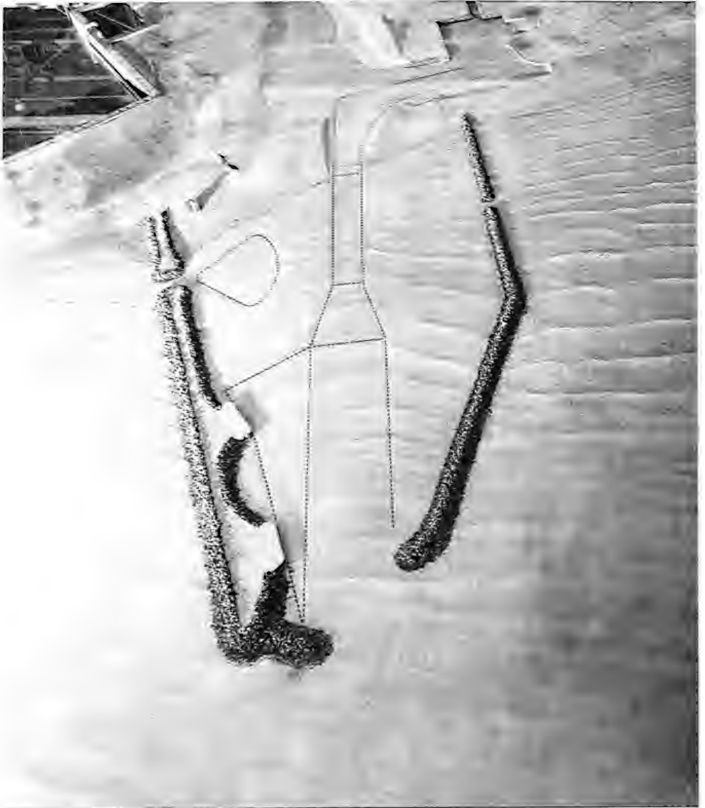
Photo 1. Typical wave patterns for Plan 19; 9-sec, 2-m (6.6-ft) waves from 227 deg, swl = +0.5-m (+1.6-ft)
