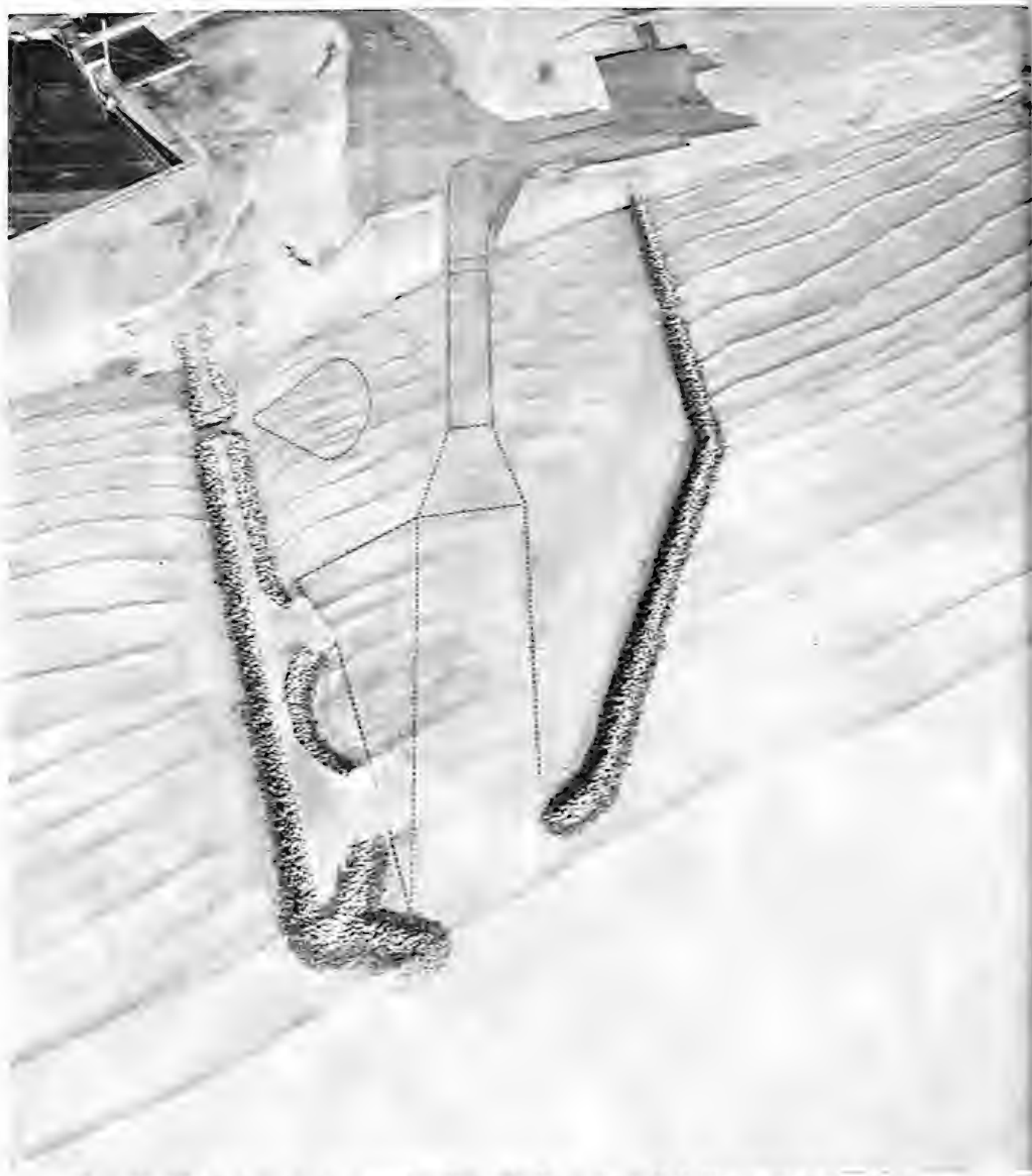
Photo 4. Typical wave patterns for Plan 19; 9-sec, 2-m (6.6-ft) waves from 182 deg; swl = +0.5-m (+1.6-ft)
