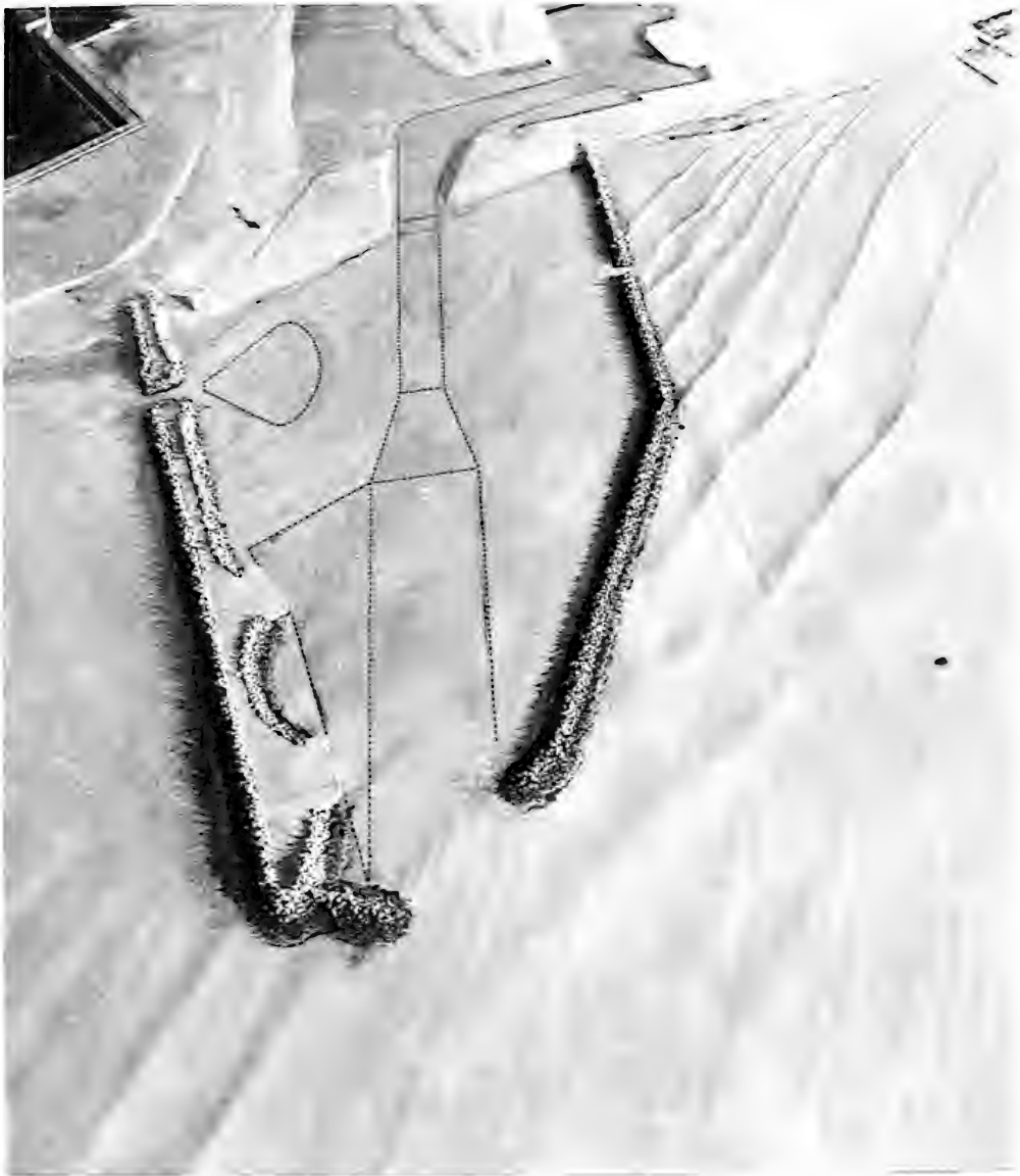
Photo 8. Typical wave patterns for Plan 19; 12-sec, 1-m (3.3-ft) waves from 137 deg; swl = +0.5-m (+1.6-ft)
