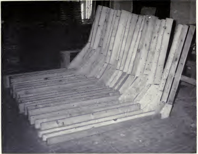
Twenty-two different types of joints were tested. Twenty-one are shown here. (Fig. 3)
