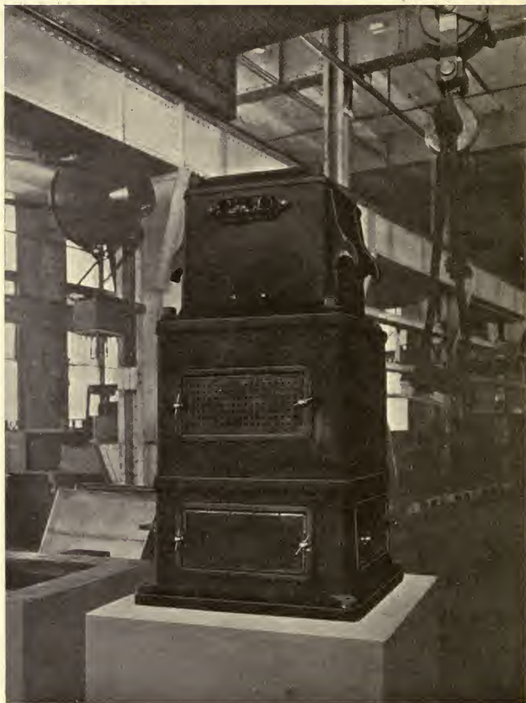
FIG. 92.—550-kva 50-cycle air-blast transformer by the Westinghouse Co.
