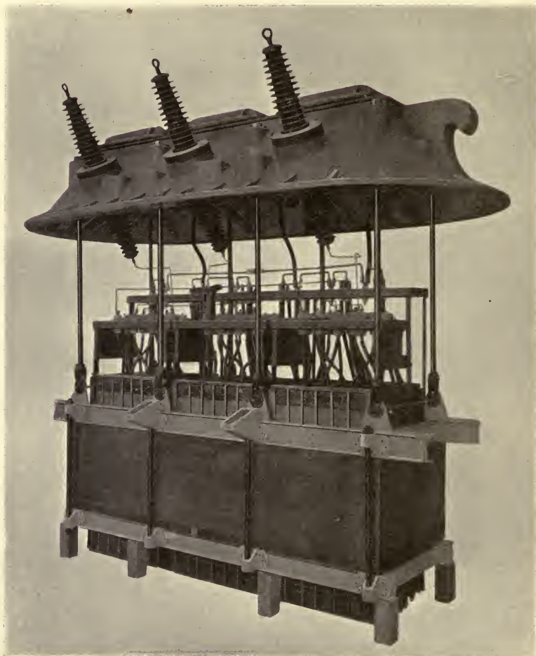
FIG. 96.—View of the interior of the American General Electric Co.'s 10 000-kva 100 000-volt 60-cycle design for a water-cooled oil-immersed transformer before the cooling coils have been mounted.
