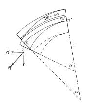
The above figure is a side view of a portion of an arcording contained between two planes perpendicular to the neutral surface non' and making an angle  $\infty$  in circular measure, before strain, between them. A vertical plane midway between the faces of the arch intersects the neutral surface in the line non' =  $\Delta s$  feet in length, which may be called the neutral line. The forces considered all act in this plane.
