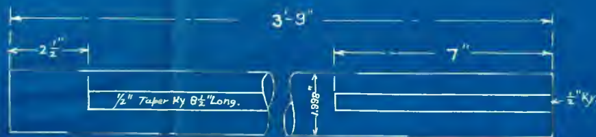
T-162 Belt Pulley Shaft .45 Carb Steel. 1- Reqd.
