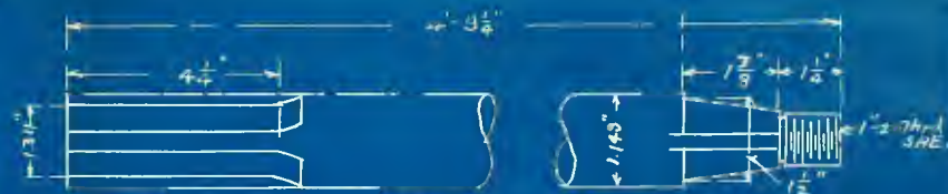
T-161 Belt Drive Shaft. .45 Carb Steel Case Harden. 1- Reqd.
