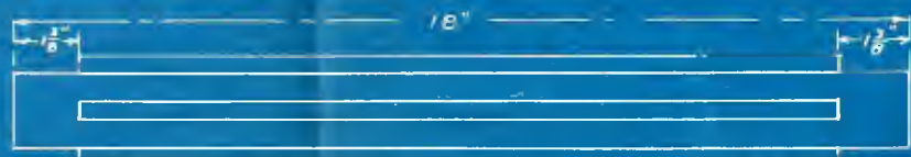
T-158. Counter Shaft. .35 Carb St. Case Harden. 1- Reqd.
