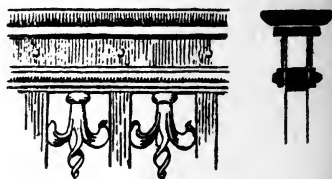
No. 150. Wrought Iron Built-up Mouldings.
