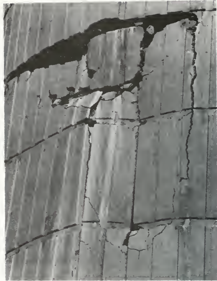
Photo 1-3 Detailed view of imploded section. (SOUTHAMPTON)
