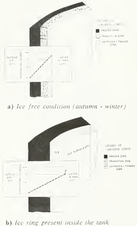
Figure 3.8 Typical seasonal wall conditions
