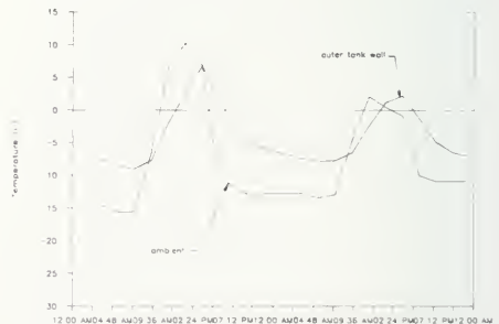
Figure 3.11 Daily temperature cycle showing daily freeze-thaw cycles at the South side of the tank
