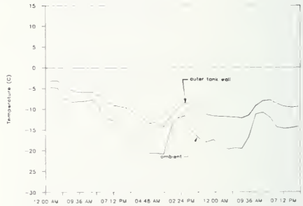
Figure 3.10 Daily temperature cycles showing continuous freezing at the North side of the tank
