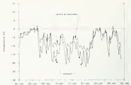
Figure 3.4 1984 winter data on north side of an uninsulated tank (ROCKWOOD)
