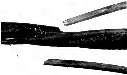
Photo 6-3 Typical longitudinal fracture of one of the wires of a strand. Lower break shows some elongation which was not typical of breaks observed. Some grease is present on the wire. (BRIGDEN)
