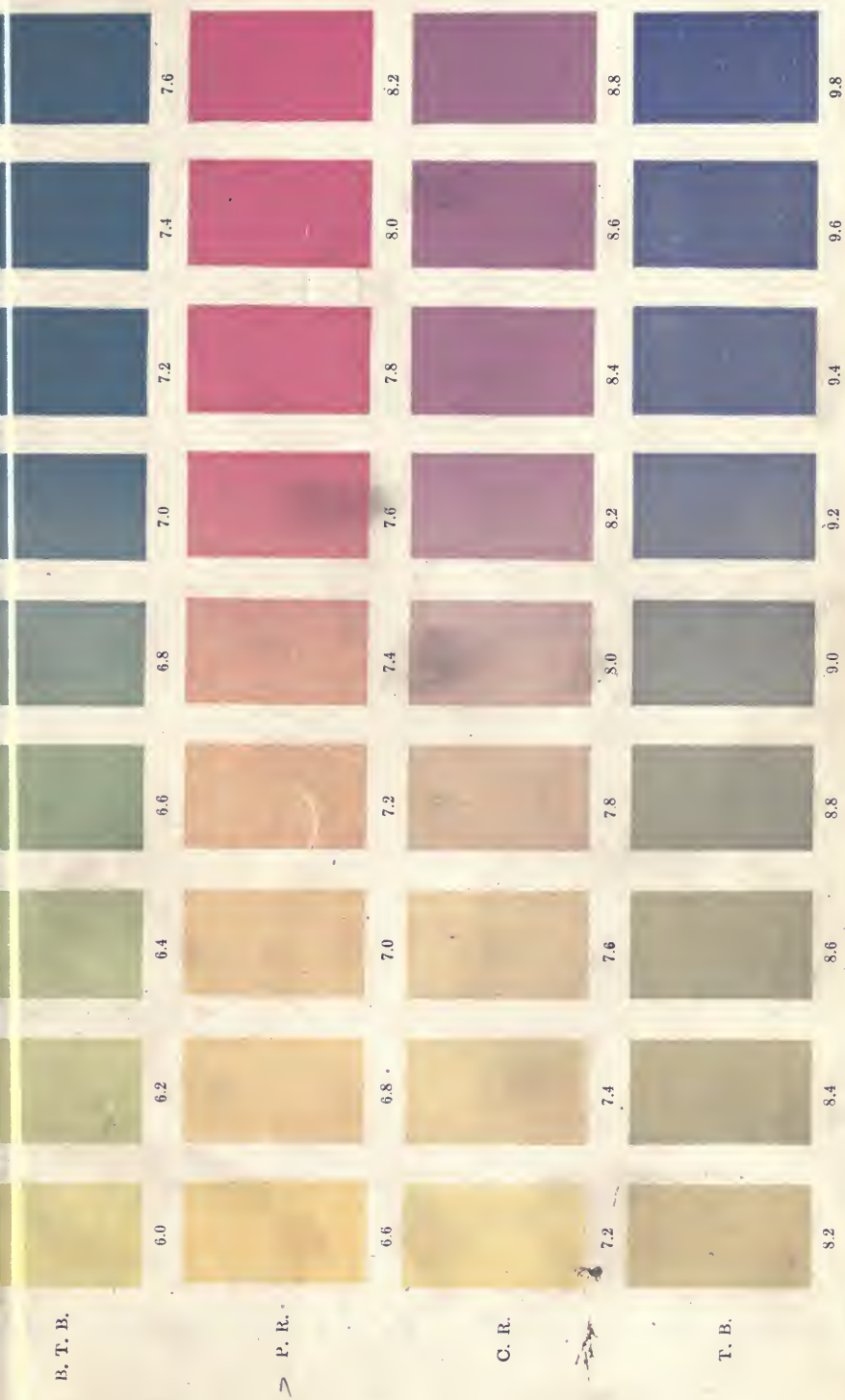
FIG. 8. CHART SHOWING THE COLORS OF CLARK AND LUBS' INDICATORS IN SOLUTIONS OF KNOWN pH
