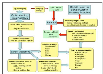
**Figure 1**: Flow diagram illustrating technologies and capabilities required to fulfill the objectives of a sample return mission.
