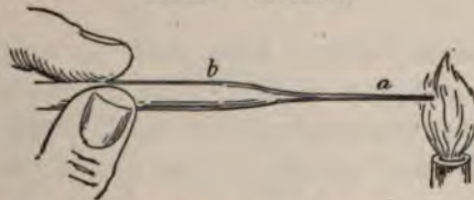
FIG. 261.—Rounding off the rough edges of the glass in the flame. (Ashton.)
