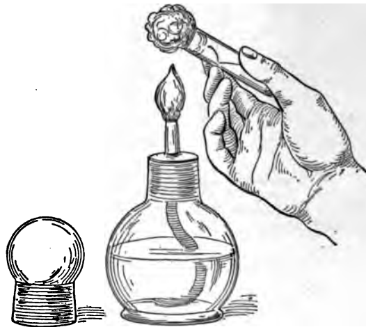
FIG. 250.—Singeing the cotton stopper of a culture tube preparatory to its inoculation.
