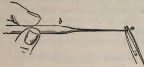
FIG. 260.—Snipping off the fused point of the slender end (a) of the pipette with scissors. (Ashton.)
