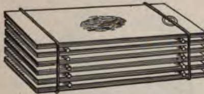
FIG. 238.—Glass slides separated by match sticks and held together with rubber bands ready for shipment to the laboratory. (Ashton.)
