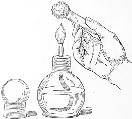
FIG. 223.—Singeing the cotton stopper of a culture tube preparatory to its inoculation.
