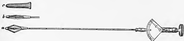
FIG. 614.—Otis' urethrometer. a , Instrument open; b , instrument closed; c , rubber stall to cover the end of instrument.
