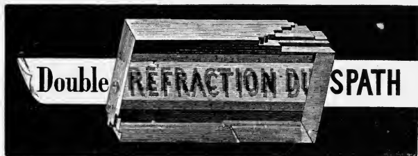
Fig. 17.—Double refraction of Iceland spar.
