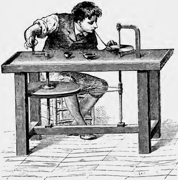
Fig. 125.—Apparatus for Sawing Hard Stones.
