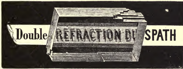
Fig. 17.—Double refraction of Iceland spar.
