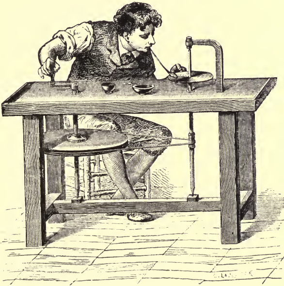
Fig. 125.—Apparatus for Sawing Hard Stones.
