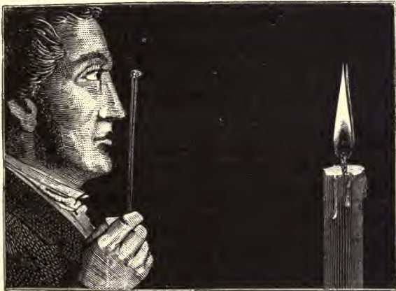
Fig. 18.—Aspect of a candle seen through a doubly-refractive crystal.
