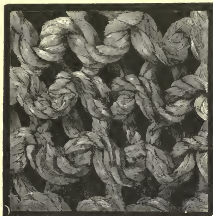
FIG. 2.—COTTON MANTLE BEFORE BURNING OFF.
