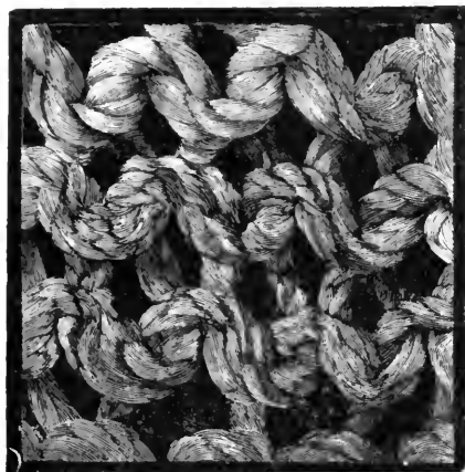
FIG. 2.—COTTON MANTLE BEFORE BURNING OFF.
