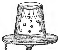
DANCING PITH BALLS. An experiment illustrating electrical attraction. It is per-
