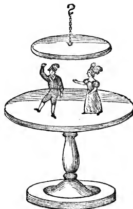
DANCING PITH BALLS. An experiment illustrating electrical attraction. It is per-
