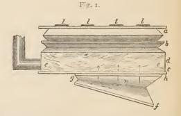
The top board a is substantially and strongly made of pine, ledgered at each end, or in large bellows panelled; some of the panels being moveable allow easy access to the interior for repairs. The middle frame b is merely a surrounding frame of wood to which is attached the lower edge of the upper ribs and the upper edge of the lower ribs. The middle board c is slightly larger than the topboard, and on it rests a strong ridge d called
