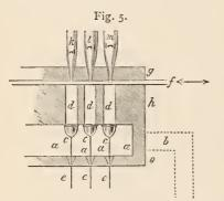
The above figure (Fig. 5) represents a section of a sound-board and wind-chest viewed from front. a is the wind-chest into which compressed atmospheric air has been introduced either through the side or bottom, from the end of the wind-trunk b. The pallets c c c are held tightly against the openings d d d, leading from the wind-chest to the mouth of the pipes by springs underneath them, thus:
