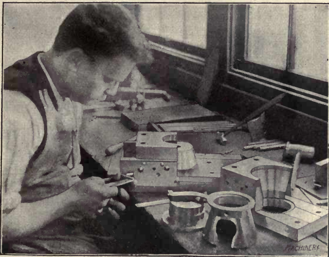
Fig. 42. Assembling a Die-casting Mold
