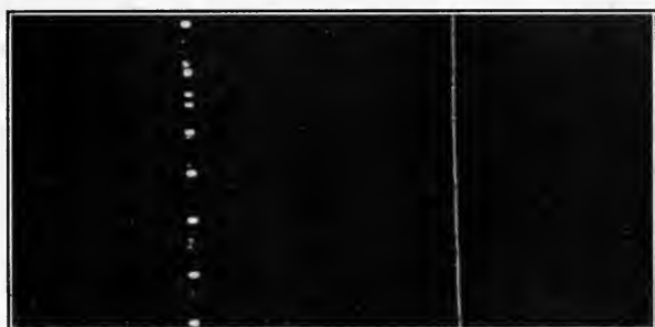
FIG. 23.—A. C. corona on polished parallel wires.
