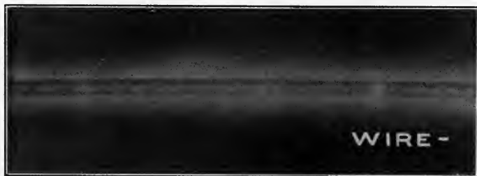
FIG. 25.—D. C. corona on smooth wires by Watson. (See Fig. 79.)
