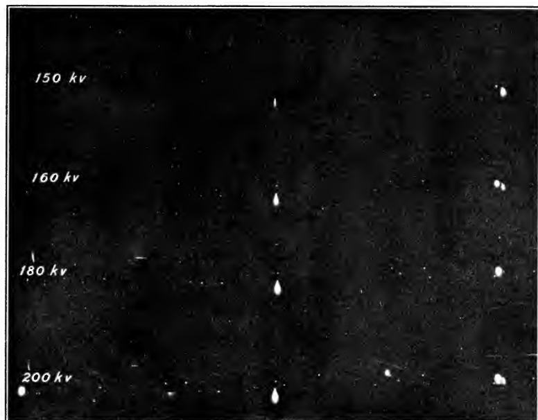
FIG. 66.—Corona on a No. 3/0 weathered cable. (Following Fig. 64.)
