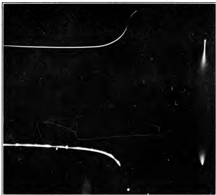
Fig. 76.—Comparison of — and \pm A. C. corona on wire and points. (Same as Fig. 75 with stroboscope.) (Following Fig. 74.)
