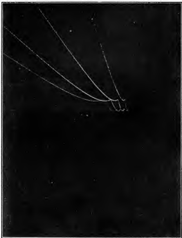
FIG. 165.—Corona at 230 kv. Line A. 3/0 cable. 310 cm. (122 in.) spacing. (Facing page 200.)
