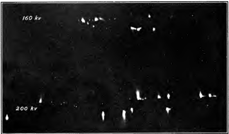
FIG. 68.—Corona on a No. 3/0 line cable. Wet. (Facing page 75.)
