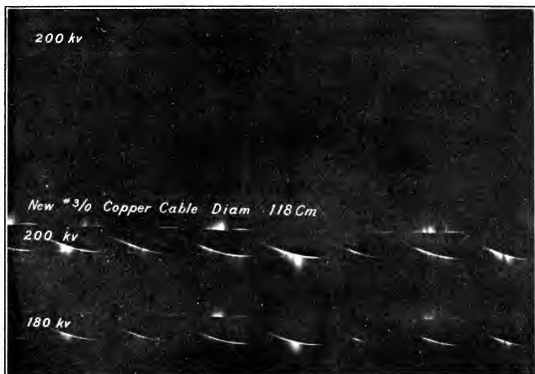
FIG. 65.—Corona on a 1.25 cm. polished brass rod and unpolished copper cable.
