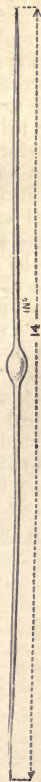
FIG. 5.—A CAPILLARY PIPETTE, DRAWN OUT INTO FINE POINTS: LENGTH ABOUT 12 TO 14 INCHES.
