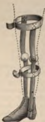
FIG. 191.—New York Orthopaedic Hospital Brace for Knock-knee and Bow-legs.
