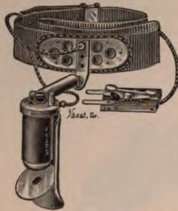
Fig. 8.—Electric head-lamp (after Kirstein).
