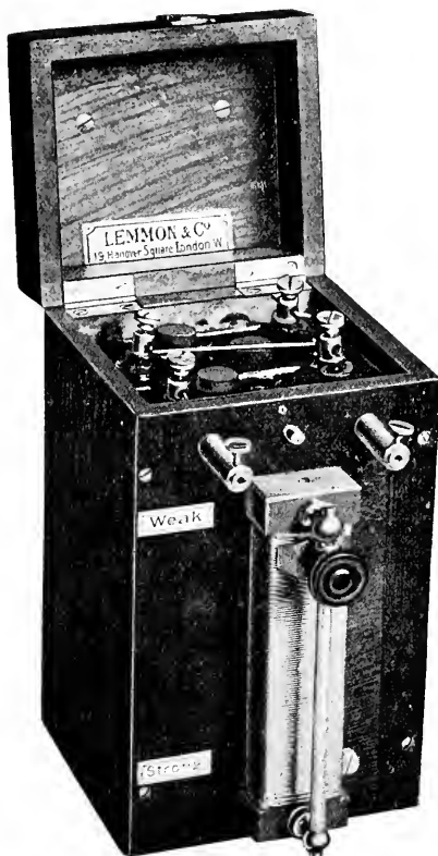
Fig. 16.—A portable accumulator fitted with a rheostat for working the sigmoidoscope.
