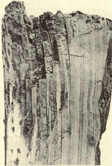
FIG. 119.— Polyporus sulfureus . Block of white spruce wood showing injury caused by this fungus. (After Schrenk.)
