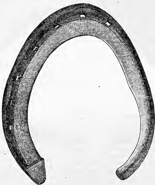
FIG. 14.—Ground surface of shoe shown in the previous figure. The inner nailless branch has the thickness of the outer branch plus its calk, so that the inner and outer quarters of the hoof are equidistant from the ground.
