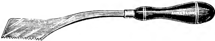
Fig. 144.—Smith's Side-bone Saw (Early Pattern).
