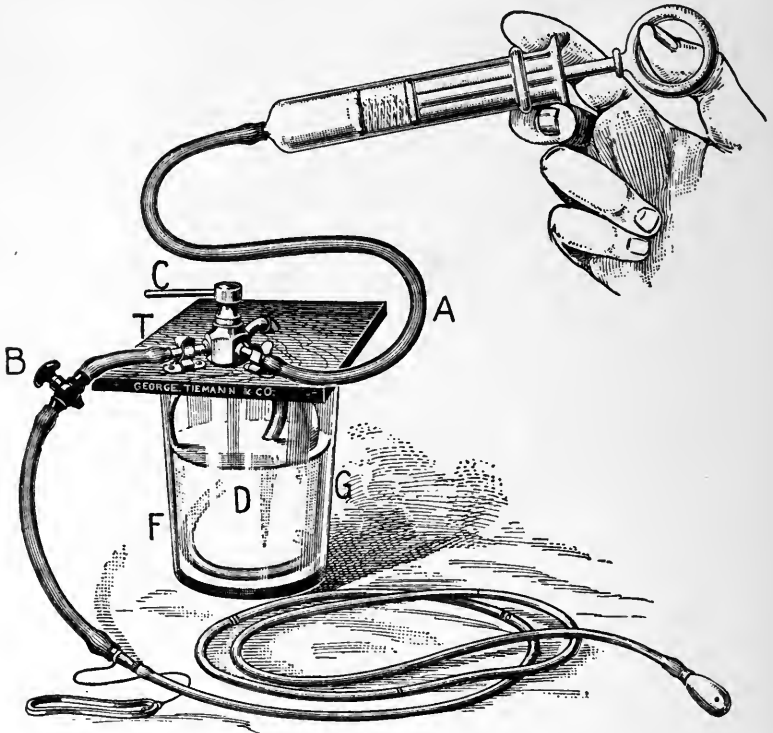
FIG. 85.—The Duodenal Feeding Apparatus, with Table Support. A, tube leading to syringe; B, tube leading to duodenal pump; C, crank; D, tube leading to fluid; F, fluid; G, glass; T, table support or shorter support. When crank C is turned parallel to A, fluid can be aspirated from the glass into the syringe. When C is moved parallel to B, the fluid from the syringe can be emptied into the duodenum.
