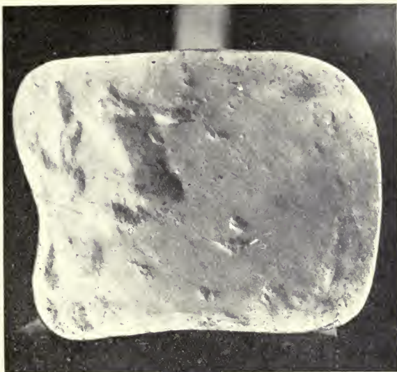
FIG. 682.—Negative Wax Cast of Electrolytic Pitting on 14-inch Cast-Iron Main.
