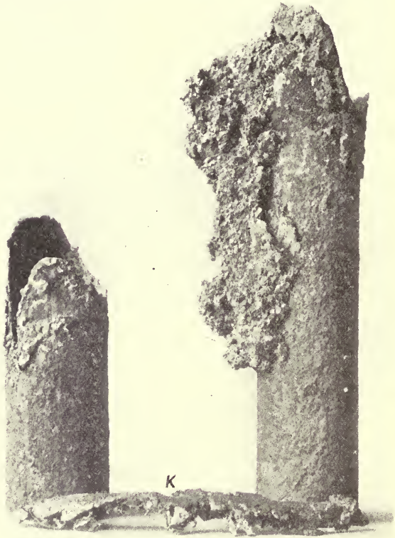
FIG. 675.—Fused portions of 2-inch Wrought-Iron Tubing, to larger scale, in which the Tram Cable was laid.
