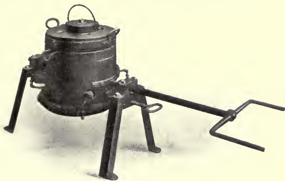
FIG. 668.—Fletcher, Russell and Co.'s Tilting Crucible Furnace.
