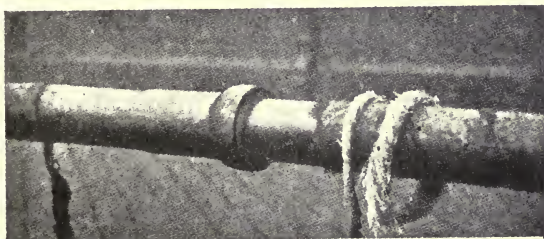
FIG. 67.—Parkinson "Rigid" Joint.
