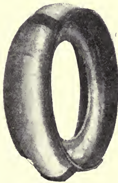
FIG. 258.—Persian Skin Stitched Diaphragm stretched on Tin Mould.
