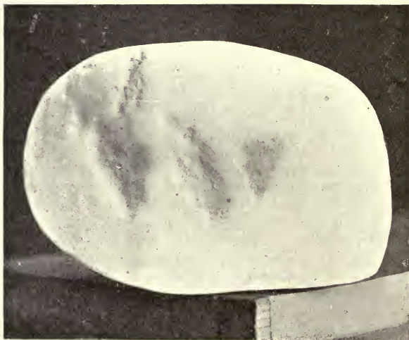
FIG. 681.—Plaster Cast of Pitting on 8-inch Main.
