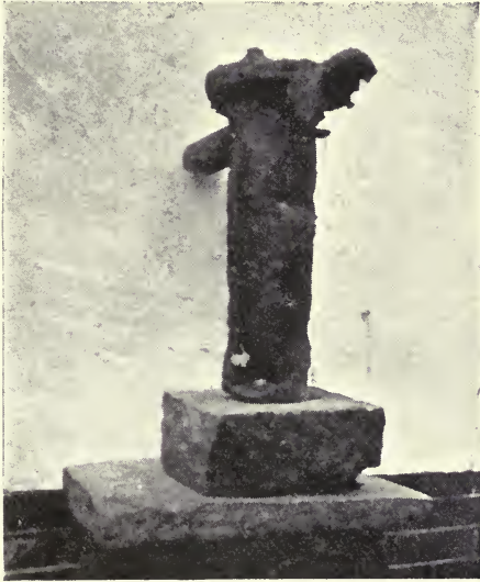
FIG. 146.—2-Inch Syphon Taken Out of Acidiferous Subsoil.
