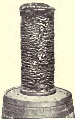
FIG. 436.—A Neglected Engine Cylinder.
