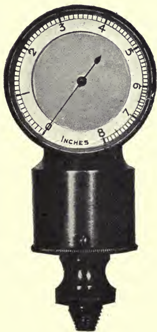
FIG. 422.—Hohmann and Maurer's Aneroid Pressure Gauge.
