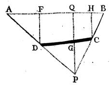
It appears, from the Corol. to the last Problem, that the tension of A D is to that of B C, as  $\frac{C G}{S. A D C}$  to  $\frac{D G}{S. B C D}$ ; whence (by the Resolution of Forces) the force of A D, in a direction parallel to the horizon, is to the force of BC, in the opposite direction, as  $\frac{C G}{S. A D C} \times \frac{S. A D F}{rad.}$  to  $\frac{D G}{S. B C D} \times \frac{S. B C H}{rad.}$ . Which forces, that the beam may remain *in equilibrio*, must
