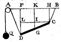
Let G be the center of gravity of the beam; also let DF, GK and CH be perpendicular to the plane of the horizon, and C L and AH parallel to the same: put-
