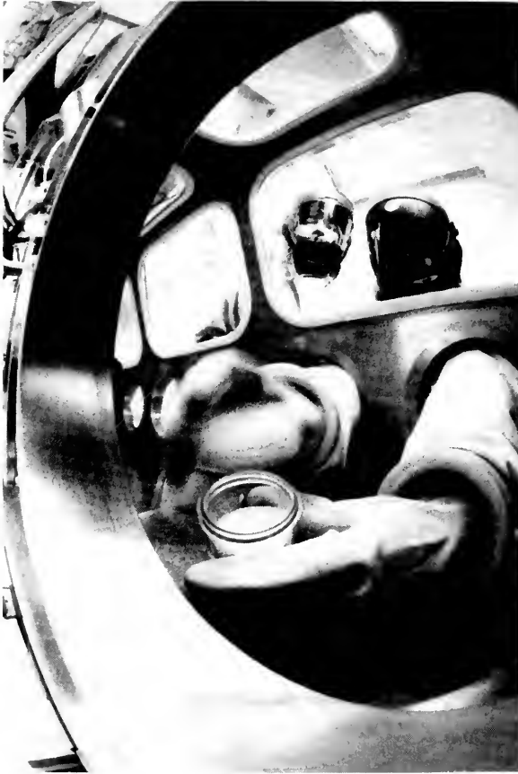
FIGURE 7-2 A group production manager (left) watches a process operator as he examines a sample of the active ingredient for PROSCAR, a drug for treating benign prostatic hyperplasia, in a sterile glove box, 1991. Source: Merck & Co., Inc., Whitehouse Station, N.J.
