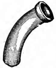
FIG. 27.—Earthenware obtuse-angle bend.
