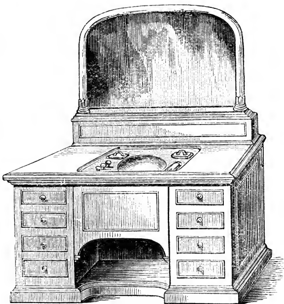
FIG. 266.—Encased lavatory for dressing-room.
