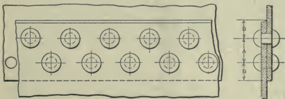
DOUBLE RIVETED LAP JOINT; EFFICIENCY ABOUT 70 %
