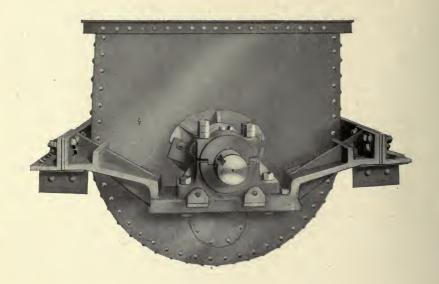
We make various sizes of these clay disintegrates from 250 yds. up to 3,000 yds. capacity per day and any number can be arranged in banks or batteries for any capacity desired.
