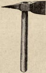
Fig. 32.—PICK FOR DRESSING AND PERFORATING TILE.
