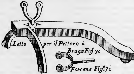
CARRIAGE OF BREECH-LOADING PIECE, SHOWING PIVOT-MOUNTING 1
